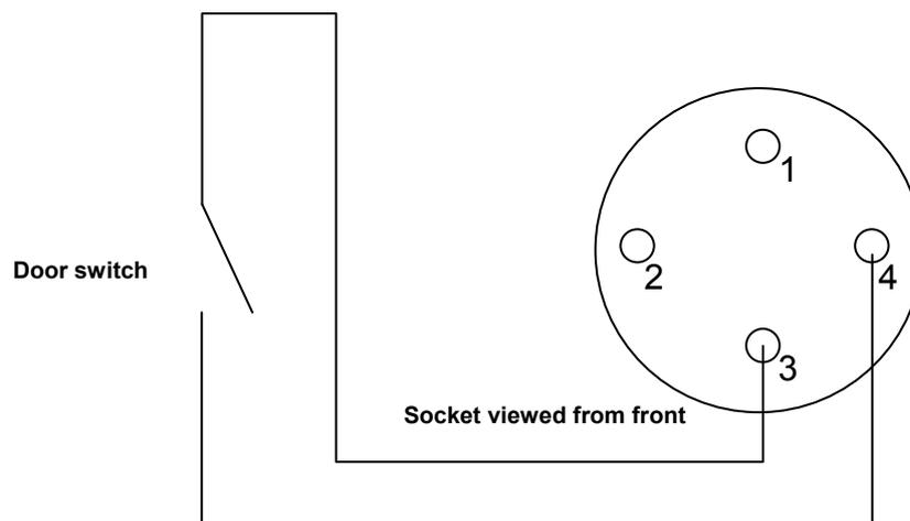
If a switch (typically a door switch) is connected across pins 3 and 4 then the module configures this as a digital input. When the switch is closed the measured input becomes a logic one, when open the measured input becomes a logic zero.
