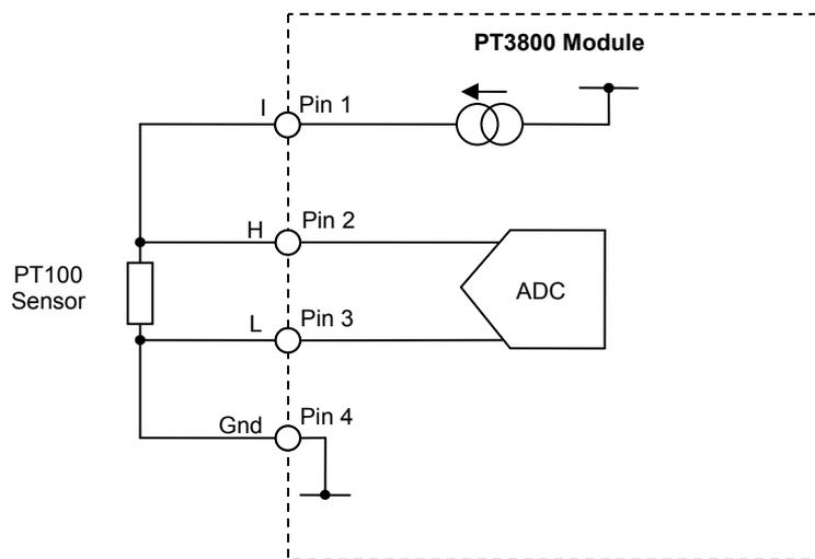
Connect a 4 wire PRT probe to any channel numbered zero thru seven. The module automatically detects that this is a PRT and configures the measurement internally.
