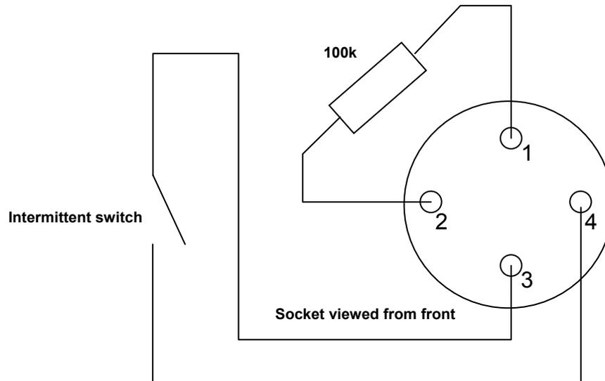
If a mercury switch (or equivalent intermittent switch) is connected across pins 3 and 4 while a ~100k resistor is applied across pins 1 and 2 then the module configures this as a motion detection input. If this input state does not change within a 30 second period, then the measured input becomes a logic zero.
